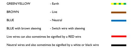
NOTE: Some luminaires may have a clear cable. In this case, the earth wire will be marked with a green/yellow thread.
