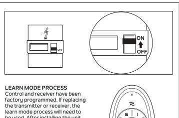
be used. After installing the unit and restoring power to your fan, press and hold the "U" button 3~5seconds. Light will flash twice and the motor spin, which indicates that the learning process has completed.
