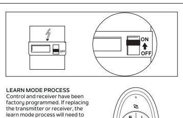
be used. After installing the unit and restoring power to your fan, press and hold the "O" button 3~5seconds. Light will flash twice and the motor spin, which indicates that the learning process has completed.
